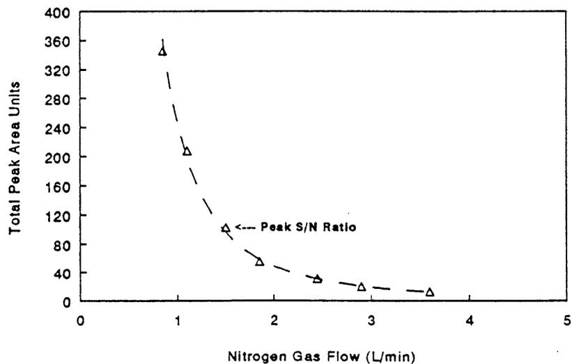
Figure 6b. Gas flow vs. peak area with the x-axis corrected for flow in liters per minute.
