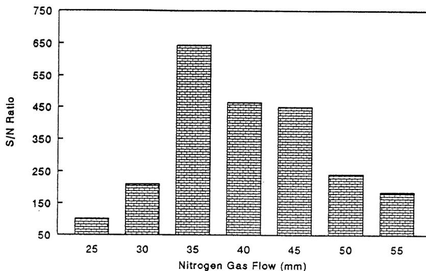
Figure 7. The above bar graph shows how the gas flow actually changes the signal to noise ratio (S/N ratio). The maximum S/N was achieved at a flow setting of 35 mm. This flow setting coupled to the optimum temperature of 120 °C should yield the highest sensitivity under these chromatographic conditions.
