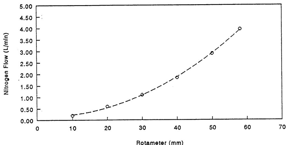
Figure 4. Mass flow calibration of the ELSD flowmeter. The conversion from 'mm' to L / min is shown.
