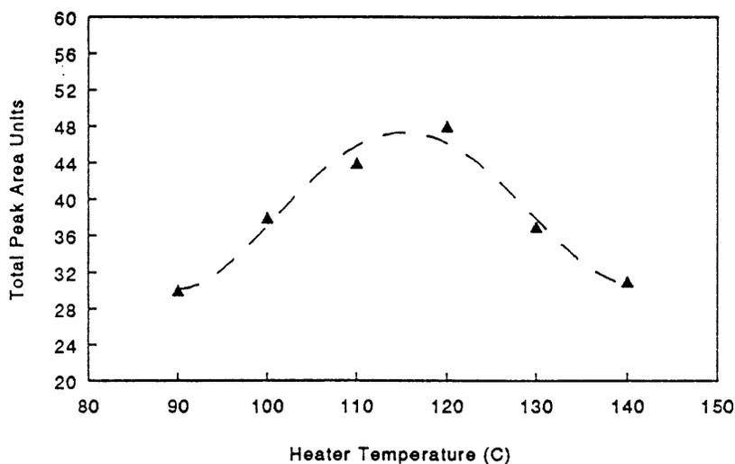
Figure 2. A Graph of the relationship between the heater temperature and the total peak area obtained. The maximum area was achieved between 115 & 120°C heater temperatures.
