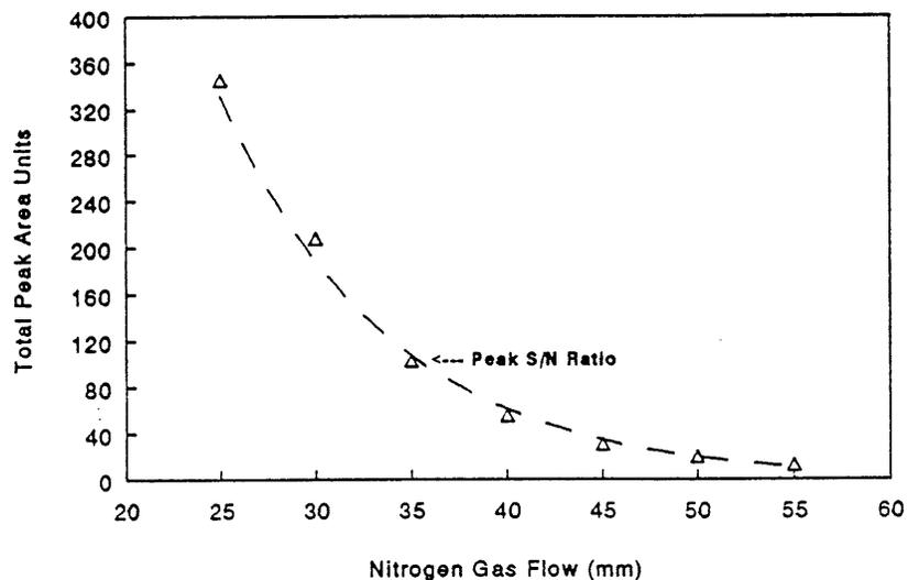
Figure 6a. The effect of varying the gas flow on peak area is shown. Note how a lower gas flow results in higher area counts while a higher flow produces a smaller area count. The optimum signal will be found at the inflection of the curve where the signal to noise ratio is highest.
