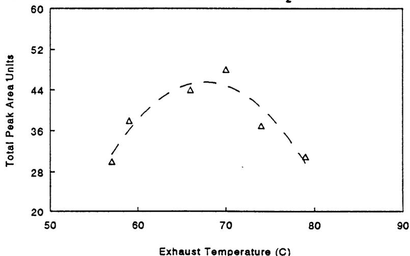
Figure 3. A plot of the detectors exhaust temperature vs. the total peak area demonstrates a maximum peak area between 67 & 70°C. This is very near the boiling point of the binary mobile phase used.
