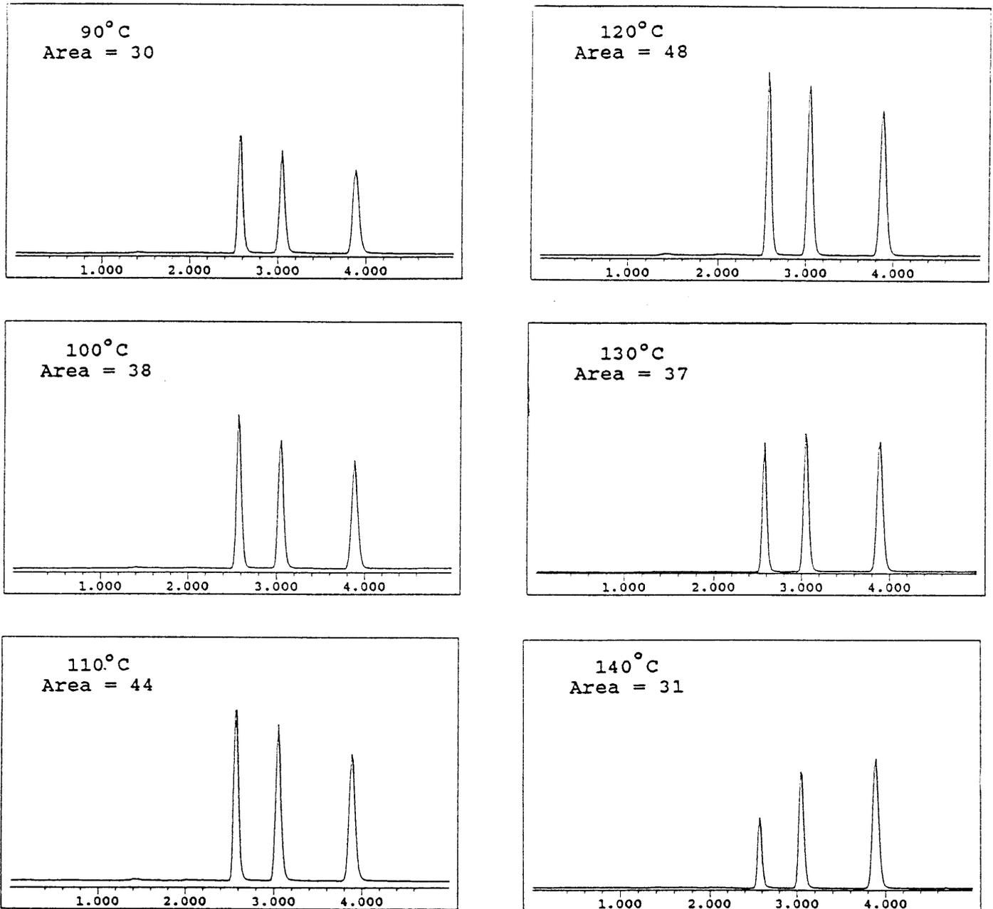
Figure 1. Chromatograms of a 3-Part standard mixture at 6 different heater temperatures selected. The results were obtained with a gas flow of 45 mm for all injections. Note how the heights and areas of the peaks change as the temperature is raised from 90°C to 140°C with a maximum at 120°C. The y-scale is the same on all of the chromatograms for comparison.
