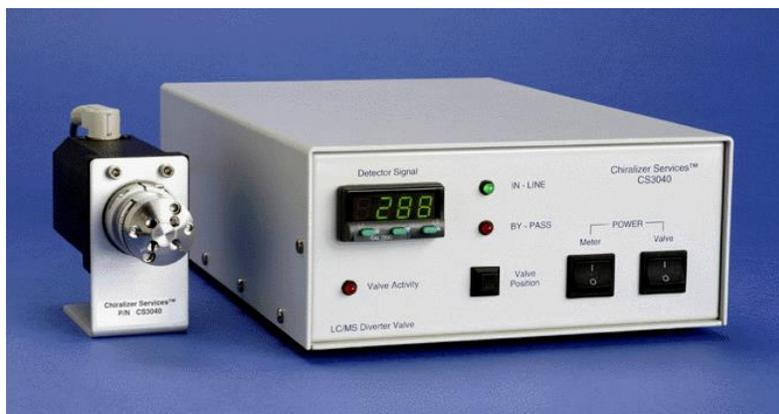
Unit includes a GLP style chart mark output for documentation purposes, a high resolution meter to monitor the detector signal input level, remote mount high-pressure SS valve (0.1 ul delay volume) as well as LED's indicating the current status. This module can be connected to most any manufacturers LC-MS system and will NOT compromise your separation.
